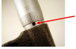
Hole that accepts wrench can be found at bottom of external cylinder.
