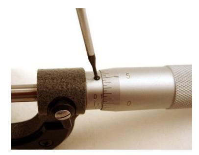
Step 5: GENTLY Open micrometer to 0.1" and tighten set screw.
